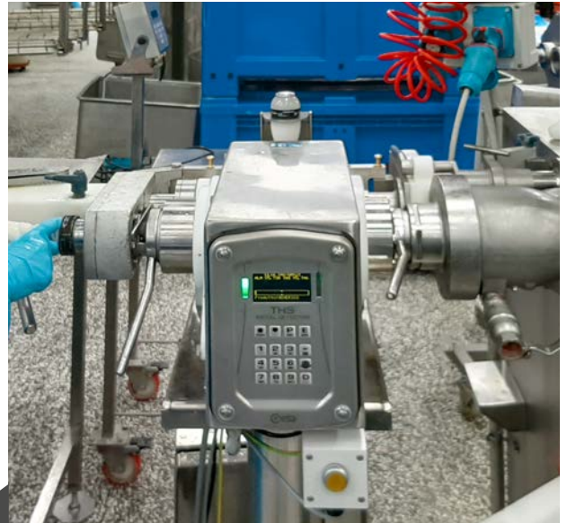
THS/PLH21 MODEL WITH INTEGRATED TWISTING EXTENSION KIT
